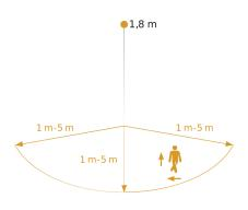
Possible mounting height: 1,80 m - 2,00 m Orange: radial and tangential 3 scalable axes
